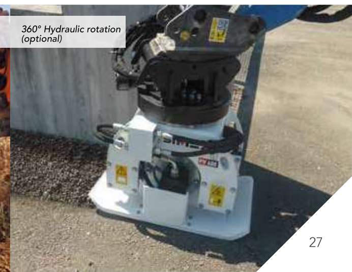
Compaction of building foundations
